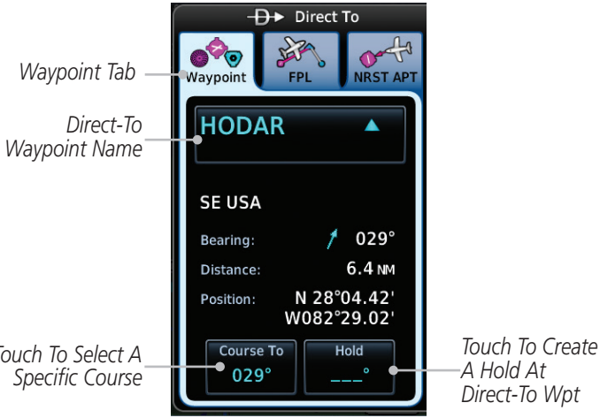
Figure 5-10 Create Hold at Direct-To Waypoint
