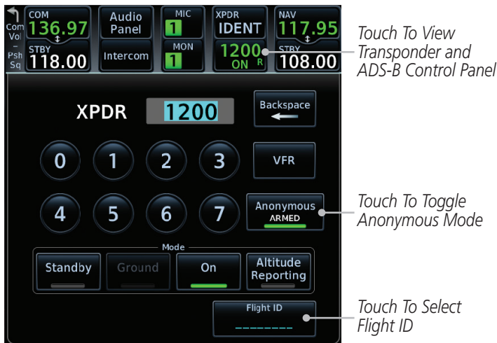
Figure 2-11 ADS-B/Transponder Control Panel
