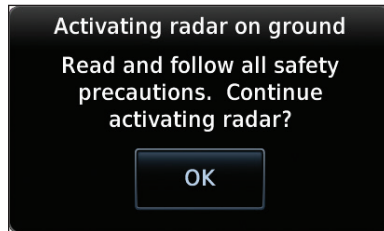
Figure 12-63 Caution for Radar Activation Confirmation
