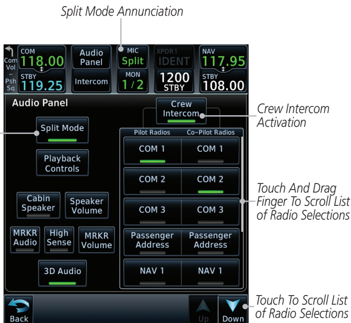
Figure 2-19 Audio Panel Split Mode Controls
