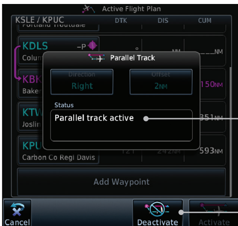
Figure 4-48 Deactivating Parallel Track
