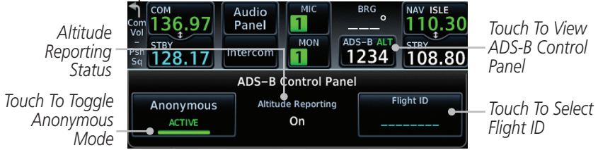
Figure 2-10 ADS-B Control Panel
