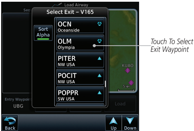
Figure 4-23 Select an Exit Waypoint for the Airway
